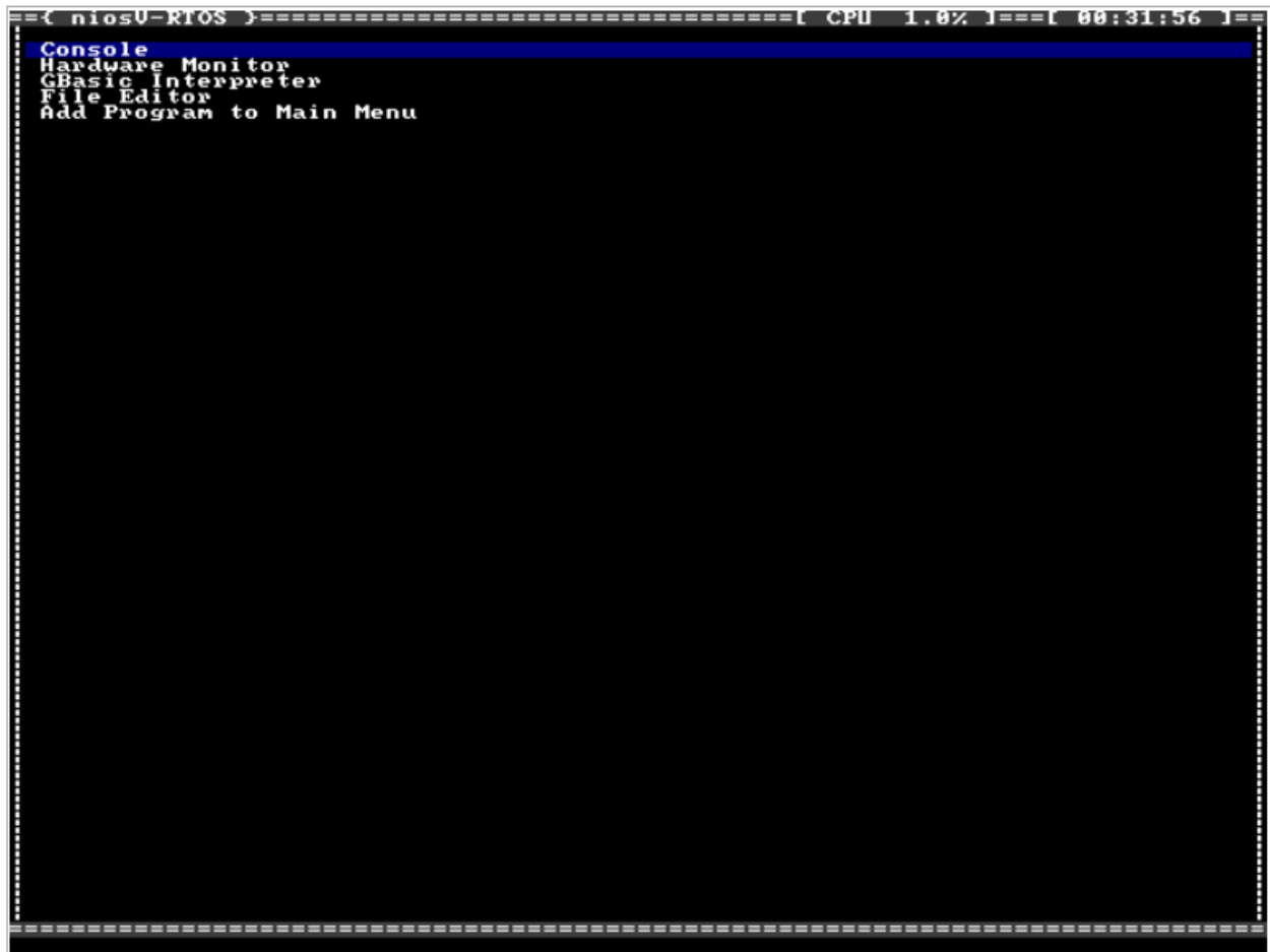
Figure 6. Shows the NiosV RTOS at initial start. The current program (i.e. Hardware Monitor, etc.) are all .gbasic scripts and are stored in the file system as <name>_native.gbasic.
